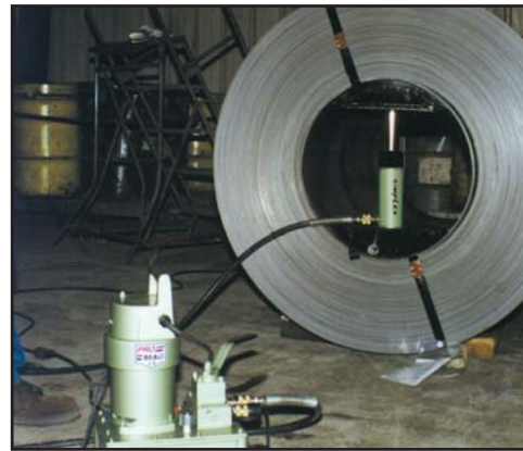
Large steel coils that were damaged in handling are reshaped using a Simplex R256 cylinder and 70 Series pump.
