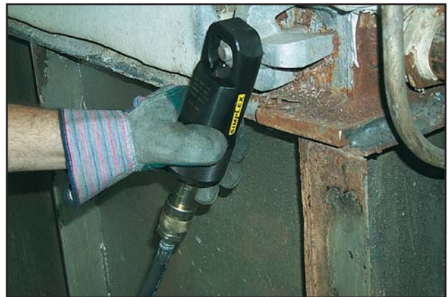
Refineries, steel mills and power plants rely heavily on Simplex nut splitters for removing stubborn or rusted nuts easily and safely. The Simplex nut splitters offer a wide range of sizes at exceptional values.
